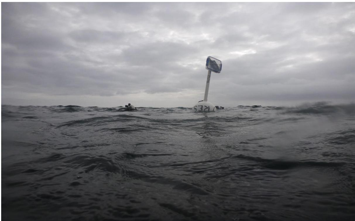
**Figure 2.** GPS unit attached to surface buoy, used to record sampling position.
